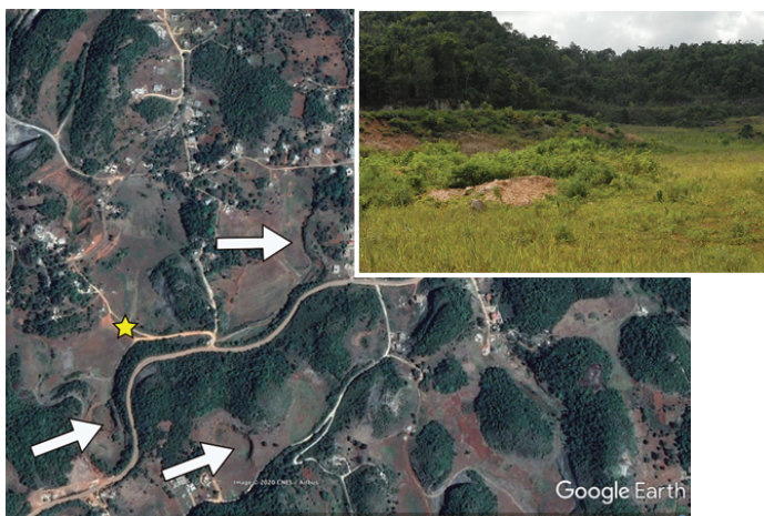
Figure 15: Vertical Scars on Hillsides from Mining and Reclamation
